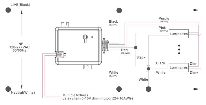
Note: BMWC-L104S MAX Load 20A, Sink Current Max.48.5mA of the dimming port. TIPS: This Bluetooth device is compatible with BlueMesh lighting control system only.
